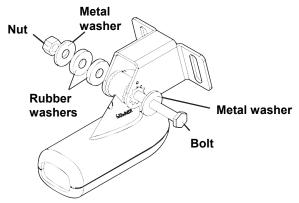
Assemble transducer and bracket.
